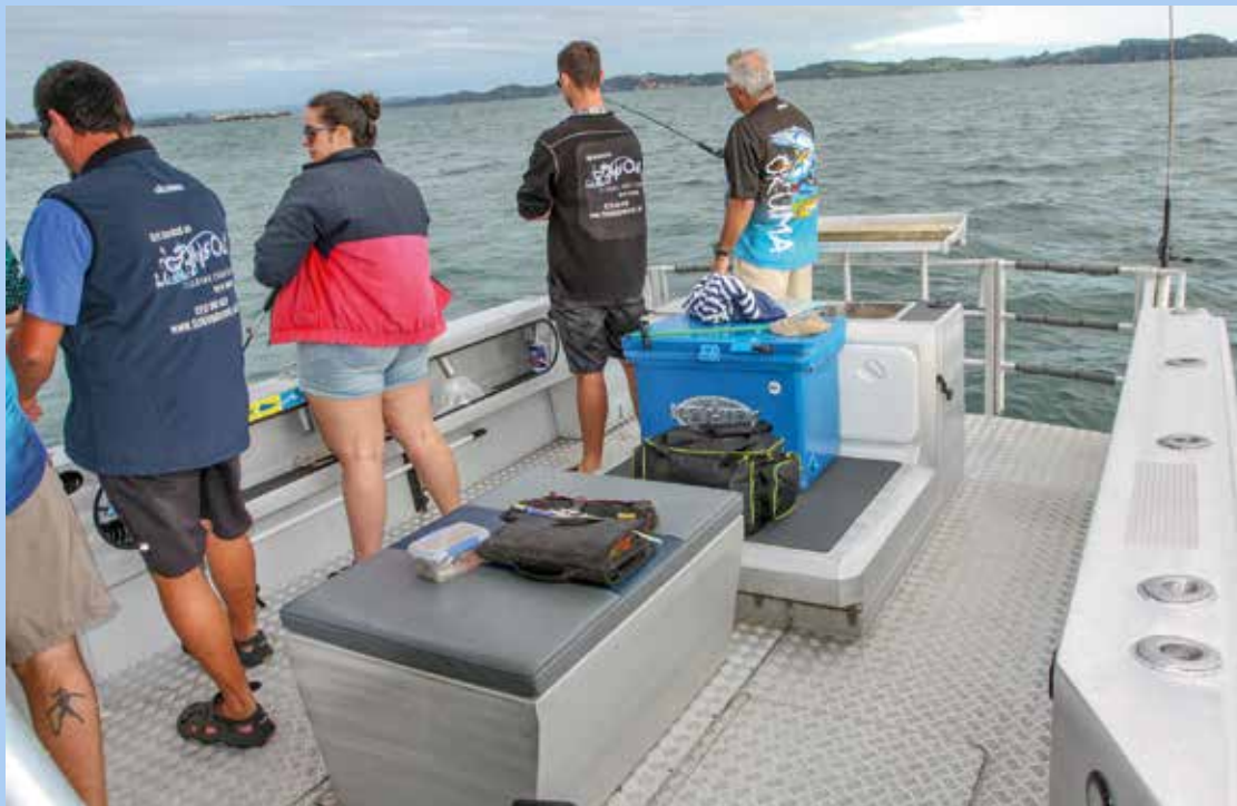
The main cockpit incorporates three kill bins below decks, a central dry storage area, Icey-Tek bin and the bait/livebait station; the helm station.
